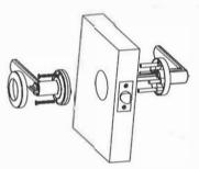
B. Insert the internal handle into position ensuring the the locking bar is located into the turn button. This can be checked by turning the turn button to ensure the it locks & unlocks the handles.
