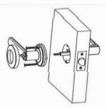
**C.** Screw both handles into position, check that the lock is working correctly and install the cover rosette.
