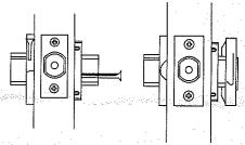
C. Install the outside escutcheon so that it sits flush to the door face. Install the inside fixing plate and fixing screws. Push on the inside escutcheon. Check that the lock functions.
