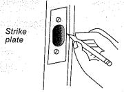
C. Alien strike plate and mark out line chisel 3mm (1/8") deep or until strike plate is flush with jamb. Chisel out behind the strike plate to accommodate nylon strike box.
