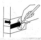
B. Mark centre hole on the door face through gulde on template for 60mm(2 3/8")backset or 70mm (2 3/4") backset.
